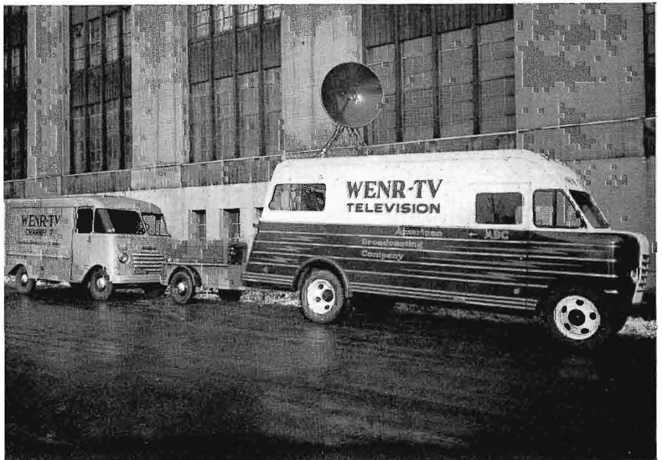
FIG. 17 (above). WENR-TV's mobile equipment includes a standard RCA TJ-50A Mobile Unit complete with portable camera equipment and RCA microwave relay gear.
