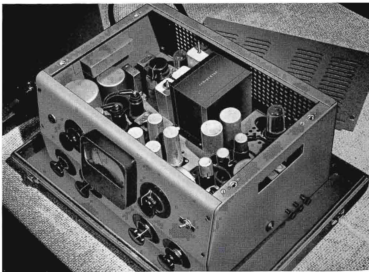
FIG. 3 (below). The RT-3A amplifier unit with top cover removed to illustrate accessibility of all parts and tubes. Note that only high-quality broadcast type components are used throughout.
