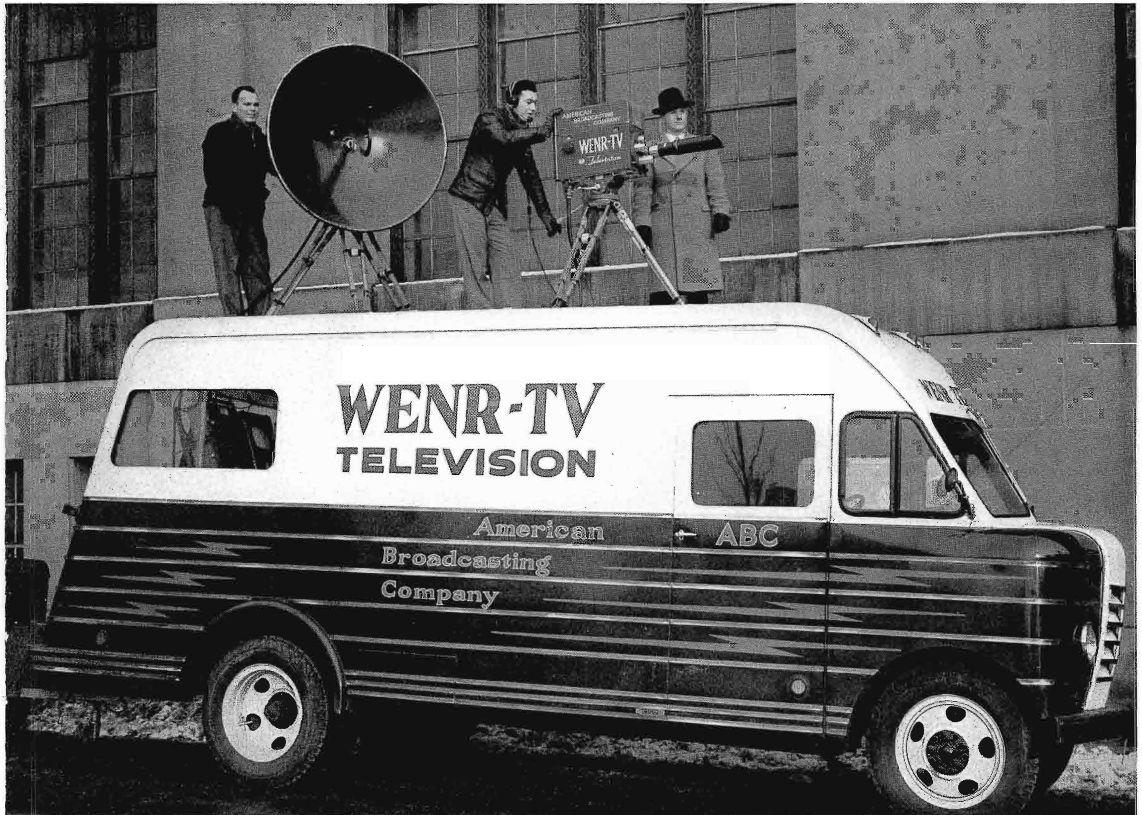
FIG. 17 (above). WENR-TV's mobile equipment includes a standard RCA TJ-50A Mobile Unit complete with portable camera equipment and RCA microwave relay gear.
