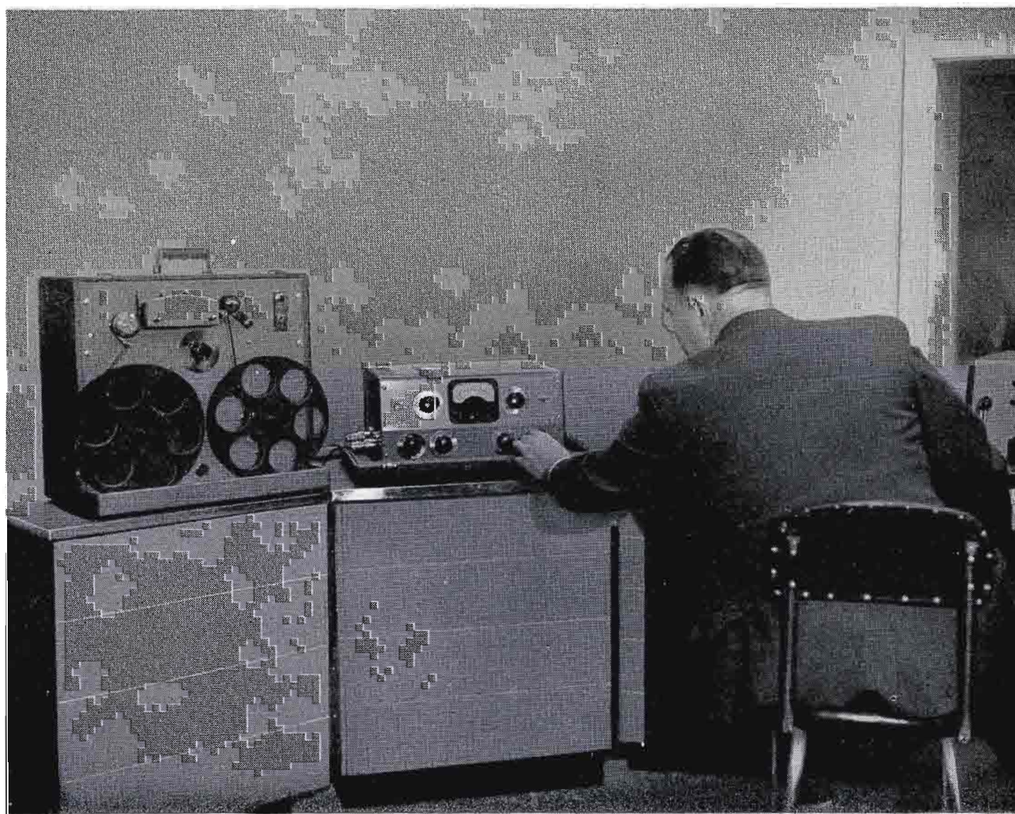
FIG. 11 (above). In this view, the operator at the console is "playing back" and putting the recorded program on the air. Note that amplifier controls, turntable and console may all be easily reached from the operator's position.
