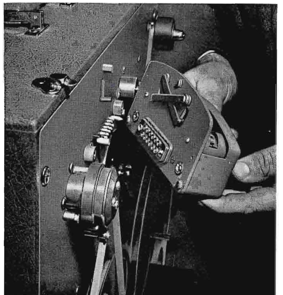
FIG. 7 (above). Threading is quickly and easily accomplished in a matter of a few seconds. Operator simply lifts tape with forefingers over the capstan, recorder heads and stabilizer in one operation.
