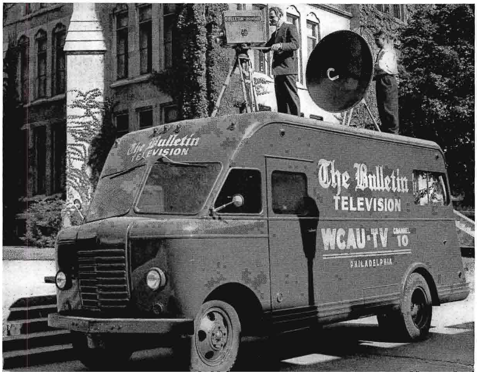
FIG. 32. WCAU-TV's Field Equipment is a standard RCA TJ-50A Mobile Unit furnished with three camera chains, master monitor, relay equipment and accessories.
