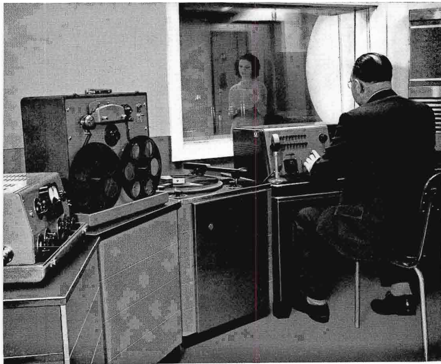
FIG. 12 (above). Here, a program originating in the studio is recorded in the control room with the RT-3A recorder. Note that cable lengths and connections permit use of various arrangements of the recorder and amplifier.
